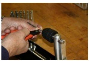
3) Remove the coiled wire from the mandrel. The end that is inserted into the arbor hole may be clipped or lifted out. Clip off or bend either end that may be sticking out above the coil. This will insure that the coil will lay flat in the V bed of the coil holder
