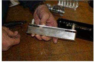
12) Place the coil holding devise with the end that the coil is on against the stop. Place the hand piece holding collar with the HP and blade in place on the coil holding devise. Run the flex shaft at full speed and with both hands and a light grip; pull the collar evenly towards you slowly. Once the cut is complete, remove the jump rings from the
