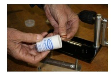
6) Place the coiled wire into the coil holding devise making certain that the lubricated side of the coil is up and the coil butts up against the stopping bracket.
