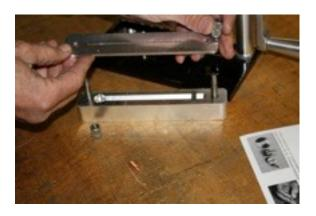
4) Remove the cover of the coil holder, be careful not to lose the springs under the cover.
