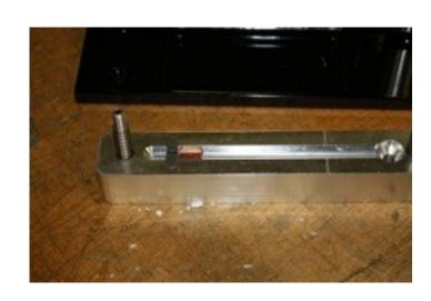
7) Place in position the 1 ¼" circular blade on the blade arbor. The name on the blade must be facing the arbor. Secure the blade arbor with the blade attached on to the No. 30 Foredom hand piece. NOTE: The 1 ¼" blade is able to cut wire gauges up to 14 gauge
