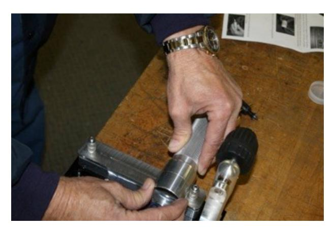
Additional mounting options - Use the included attachment to securely mount the winding coil to a sturdy surface.
